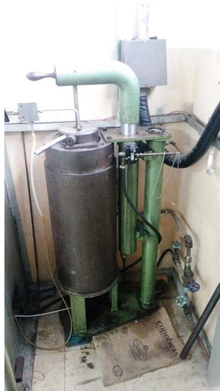
Figure 2: Isostatic press machine used for pressing of pre-compacted \text{ThO}_2 pellets.
