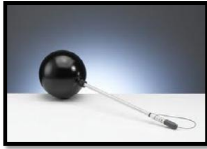
Figure 5: Ionization chambers with sensitive volume of 1000 cm 3 (model 32002).
