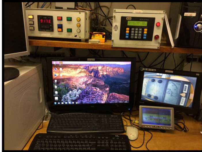
Figure 7: Control room of portable monitors calibration laboratory. Being able to see the control caesa radiator, control of automated table with their cameras to detect the reader's display and its source detector position.
