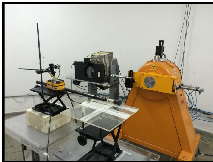
Figure 8: Irradiation Room of portable monitors calibration laboratory. It is able to view the radiators B 85/1 and Caesa, positioning table and a teletector detector.
