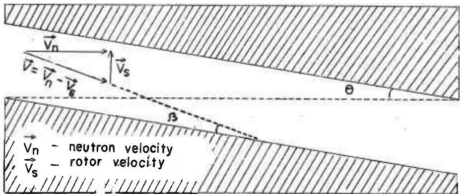
Figure 2 - Vectorial velocity composition within the channel.
