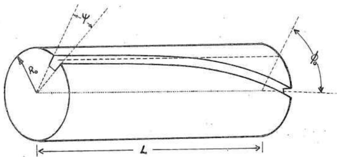
Figure 1 - Selector geometry
