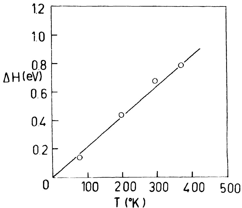
Figure 1 – Variation of activation enthalpy with temperature in LiF
