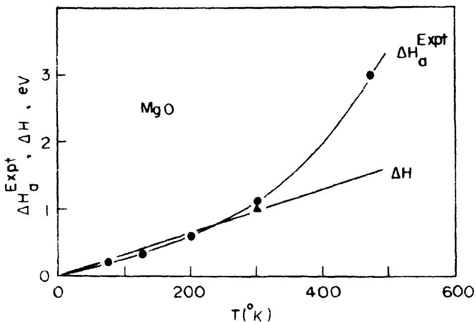
Figure 2 - Variation of activation enthalpies with temperature in  $MgO$  from refs 6,7. Observed values given by (○); corrected value at room temperature by (●) (See text)
