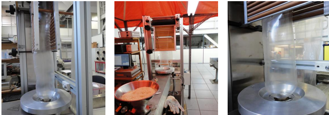
Figure 2: Extruder Haake-Rheomex device used to process the polymeric films. Polymer Laboratory at Center for Chemical and Environmental Technology (CQMA) / Nuclear and Energy Research Institute (IPEN).
