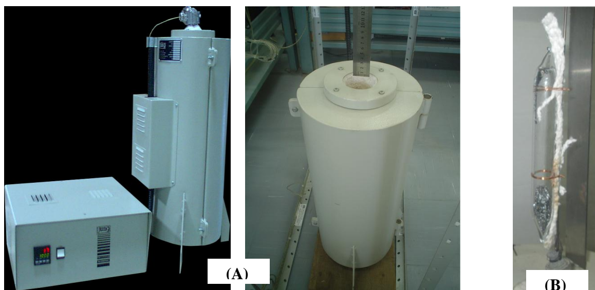
Figure 2: Vertical Bridgman Furnace used for \text{BiI}_3 purification (A) and Tube with \text{BiI}_3 (B)
