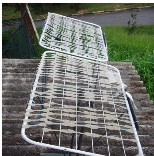
Figure 1: Device with dumbbell samples for environmental ageing outside at the IPEN/CQMA
