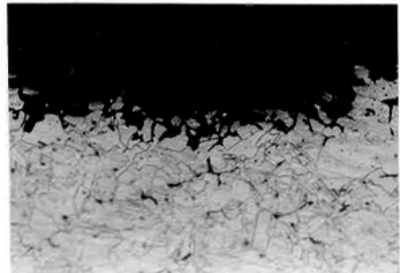
Fig. 14 - Intergranular corrosion of steel AISI 347(2) sensitized during 13 h at 790°C, after 30 min immersion in practice B testing solution. OM. Etched with oxalic acid. 150X.
