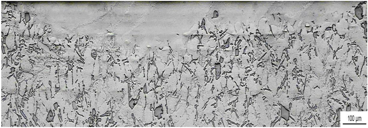
Figure 6. Optical micrograph of transversal section of Al-Si alloy sample after LASER irradiation producing track (TRL2 condition)
