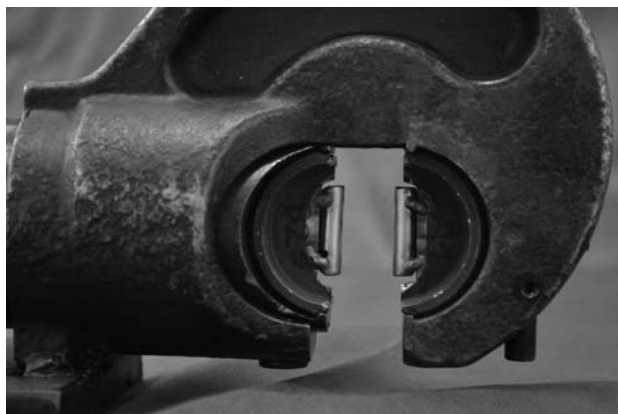
Fig. 2 Hydraulic presshead with semi-circular slotted die modified.
