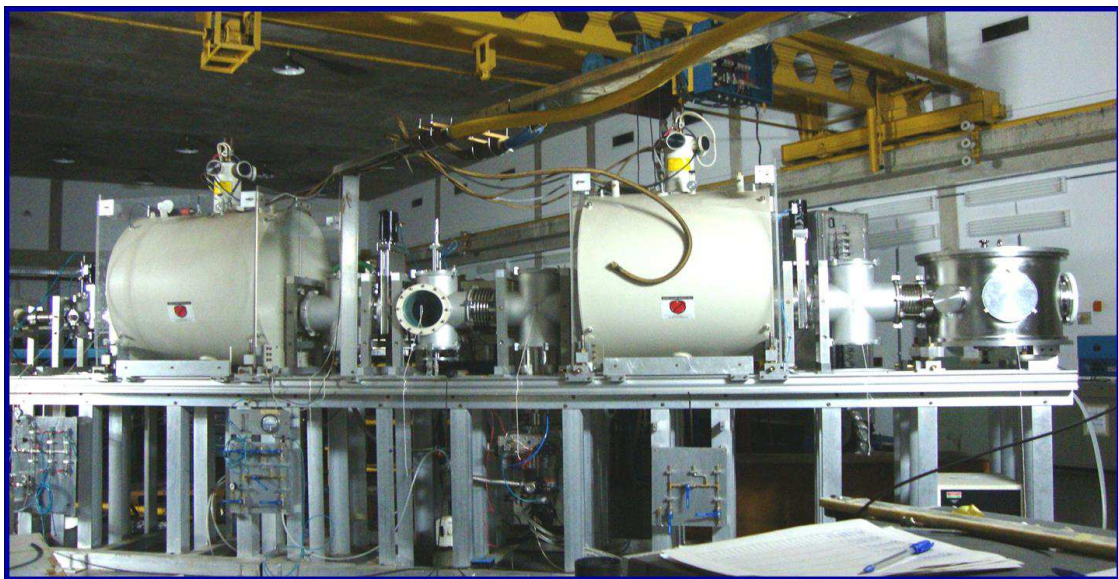
Figure 1. The RIBRAS facility. The stable beam comes from the left, the production target is located on the left side of the first solenoid. Between the two solenoids one can see the intermediate scattering chamber. At the right extremity, after the second solenoid, the new, large scattering chamber can be seen. Taken from reference [3].
