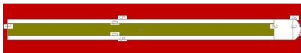
Figure 5: Design of the fourth simplification of the HDR source Varian VariSource Classic: removal of the portion of the capsule that stood between the active part of the source and the cable.
