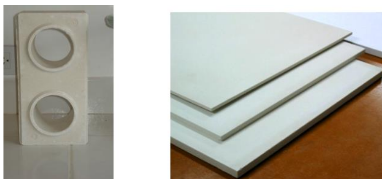
FIG. 1. Bricks and Plates made of phosphogypsum.
