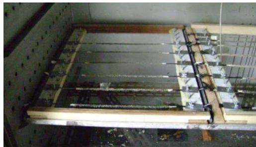
Figure 1. Rods placed in the fixation device to cure the polymer matrix.
