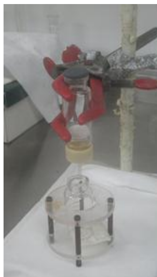
FIG. 4. Glass frit filtering device for Mo- \alpha -Bz.
