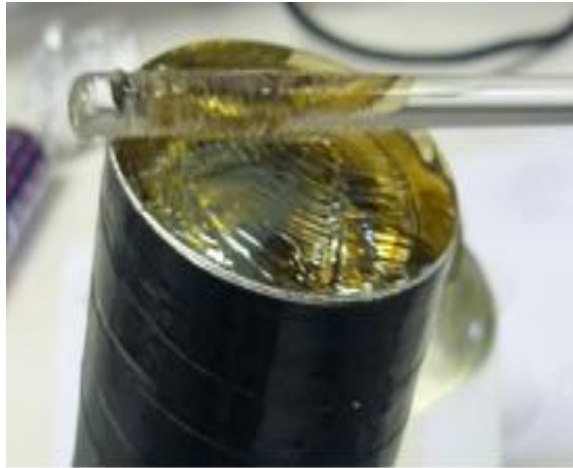
Figure 5. Optical coupling with silicon grease.
