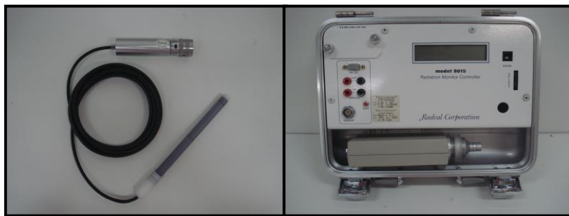
Figure 3: Pencil ionization chamber and a 9015 Dosimeter, from Radcal Corp.
