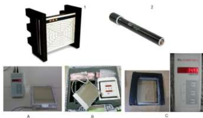
Figure 1: In 1 the Patient Dose Calibrator; 2 the ionization chamber RC6; A the KAP meter Diamentor E2; B the KAP meter KermaX plus TinO 120-205 and C another KAP meter Diamentor E2
