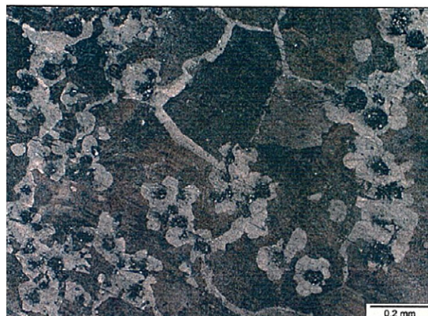
Fig. 11. Micrography obtained by metallographic replica of trunnion region. Region with light marks from Fig. 7. Zoom 100×.
