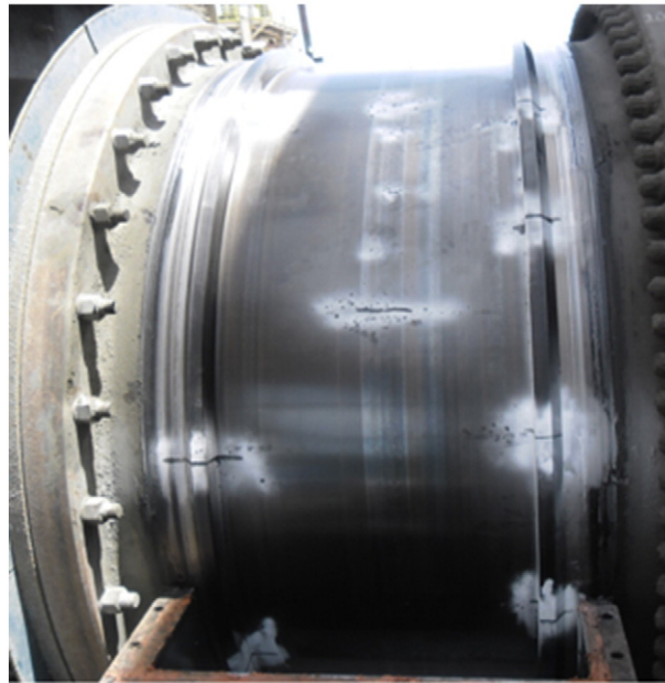
Fig. 6. Cracks location overview.
