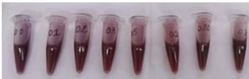
Figure 6. Gold nanoparticles irradiated for different times. From the left to the right: non irradiated and irradiated by, respectively, 1, 2, 3, 5, 10, 20 and 30 minutes.
