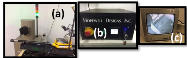
Figure 3. (a) Irradiation Room of portable monitors calibration laboratory. It is able to view irradiator Hopewell, positioning table and a teletector detector. (b) and (c) Control room of portable monitors calibration laboratory. Being able to see the control Hopewell radiator and cameras to detect the reader's display.
