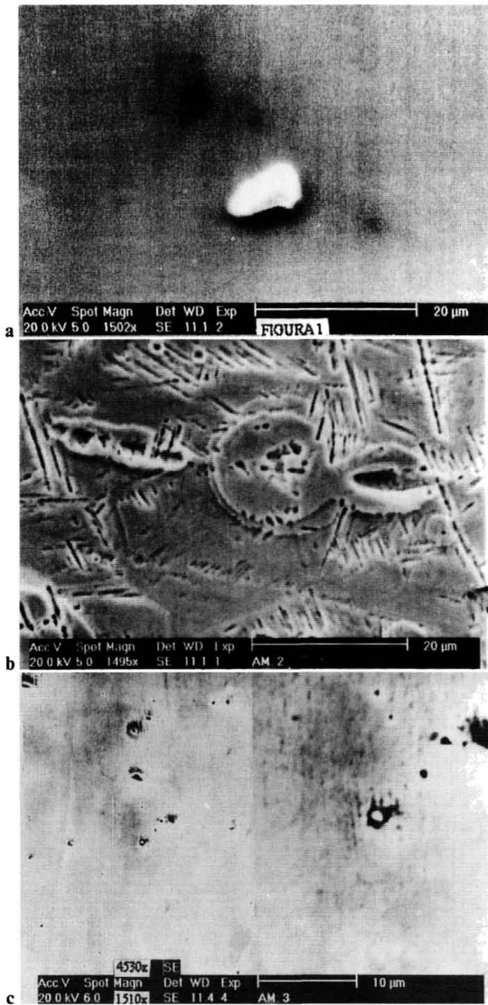
a after polishing, \times 1502 ; b after immersion in stirred 2M H_2SO_4 solution without benzotriazole, \times 1495 ; c after immersion in stirred 2M H_2SO_4 solution containing 1.0 \times 10^{-3}M benzotriazole, \times 1510 1 Scanning electron micrographs of type 304 SS
