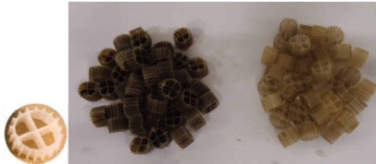
Figure 9: The small and clean biomedia applied for the biofilm improvement and the dirty used biomidias (Anox Kaldnes®), obviously related to the exposure of the biomedia to the effluent, during the treatment proposed studied.
