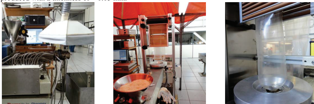
Figure 1. Extruder Haake-Rheomex device used to process the polymeric films. Polymer Laboratory at Chemistry Centre and Environment (CQMA) / Nuclear and Energy Research Institute (IPEN).
