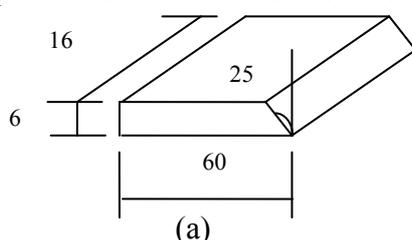
Fig. 1 - Welded samples geometry
