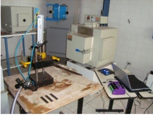
Fig. 3 - Thermal cycle reproducing equipment
