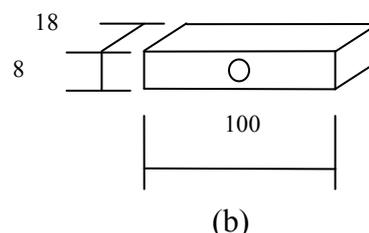
Fig. 2 - Cooling curves samples geometry
