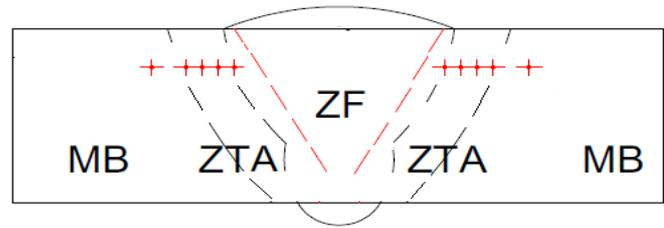
Fig. 4 - Scheme dot placement print hardness profile studied
