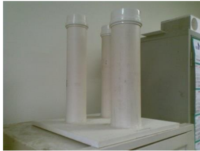
Phosphogypsum bricks and accumulation chamber / phosphogypsum plates and accumulation chamber / CR-39 radon dosimeter / Track density measurements system
