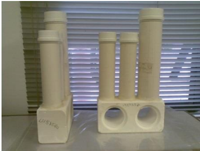
Phosphogypsum bricks and accumulation chamber / phosphogypsum plates and accumulation chamber / CR-39 radon dosimeter / Track density measurements system
