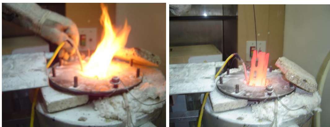
Fig. 2 Molten salt stripping—introduction (left) and removal (right) of a sample.
