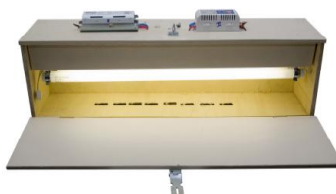
Figure 4. Homemade light box with fluorescent lamps [8].
