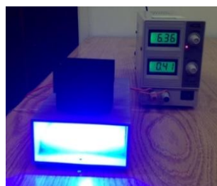
Figure 3. Homemade light box with blue LEDs.
