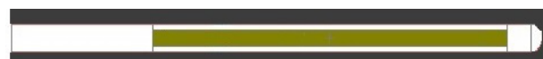
Figure 4. Design of the third simplification of the HDR source Varian VariSource Classic: removal of the stainless steel cable.
