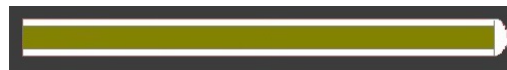
Figure 6. Design of the fifth simplification of the HDR source Varian VariSource Classic: removal the portion of nitinol.
