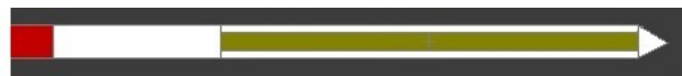
Figure 3. Design of the second simplification of the HDR source Varian VariSource Classic: replacement of the rounded tip for a triangular one.
