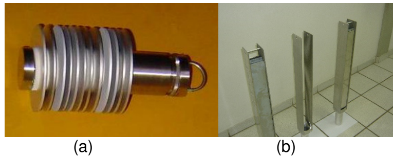
Figure 1: Photographs of: (a) coupons stacked in a rack; (b) plates assembled to form dummy fuel elements.
