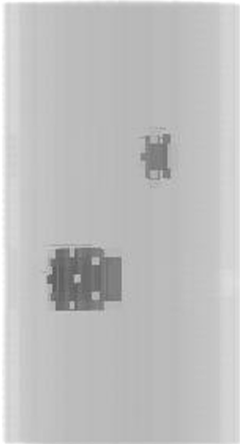
Fig. 10. 3D image reconstruction of the simulated bubbles (40 and 20 mm diameter).
