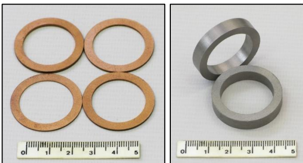
Figure 2.1: Copper rings and inserts before sintering process respectively.
