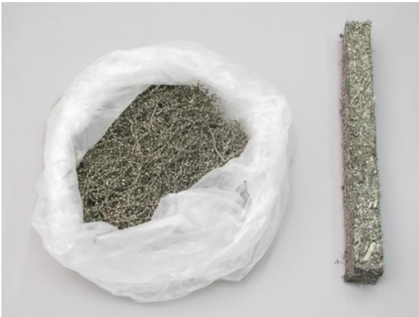
Figure 3: Clean scraps and the produced electrode.
