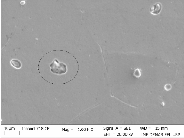
Figure 8 – SEM of Inconel 718 (as received): Details of a dark precipitate.
