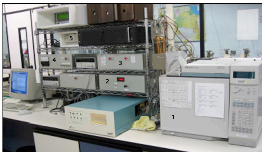
Figure 1 - GEE Analytical System of LQA / IPEN. 1: Chromatograph HP 6890 plus / ECD (Electron Capture Detector) 2: Gas flow controller; 3: Sample and system select valve; 4: Vacuum measurer and samples receiver; 5: Chromatograph's interface
