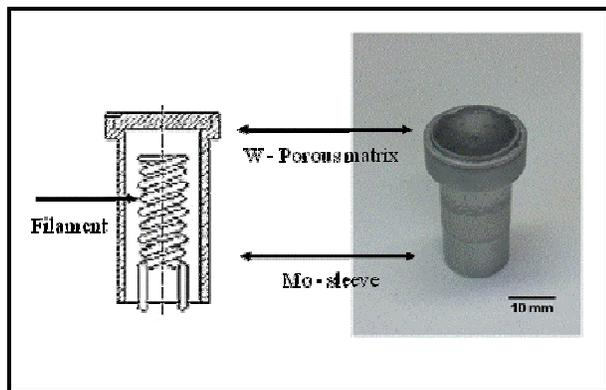
Figure 1 – Impregnated tungsten porous cathode for TWT valves.
