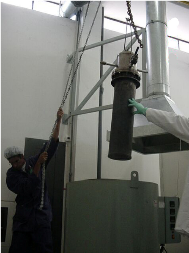
Fig. 3. Charging of the reactor vessel inside the pit furnace.
