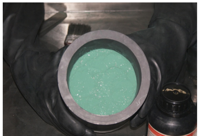
Fig. 2. View of the graphite crucible with the \text{UF}_4 + Mg load after tapping the 10 layers.
