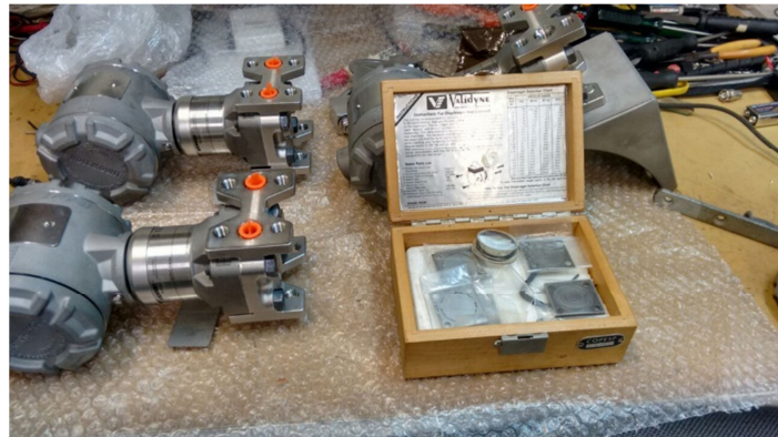
Figure 4: High accuracy reference sensor - Validyne DP15TL
