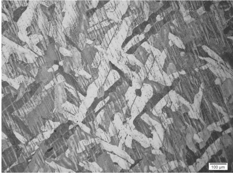
Figure 6. Zircaloy-4 microstructure sample treated with annealing showing characteristic morphology of Widmanstätten structure of basketweave form.
