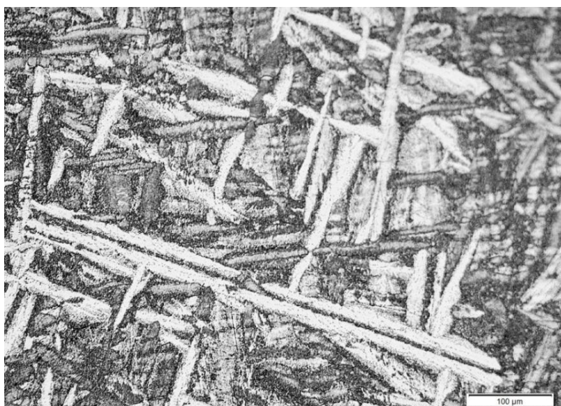
Figure 5. Zircaloy-4 microstructure obtained by the electron-beam melting method (raw state) with a Widmanstätten structure characteristic of the basketweave morphology. Etched.
