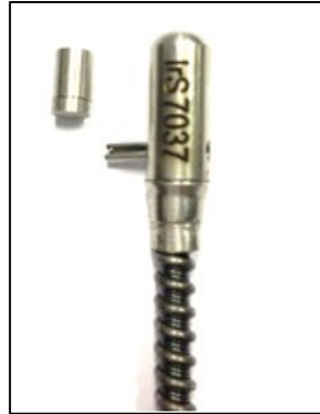
Figure 1: Ir-192 radioactive source and source holder produced at LPFS
