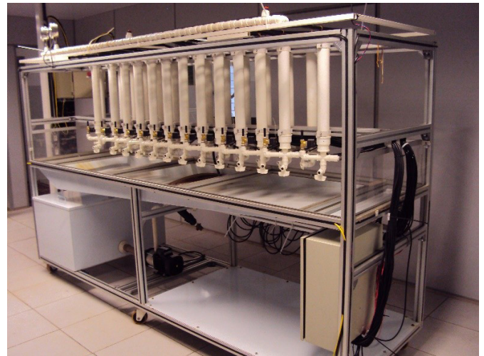
Figure 1. Test bench for determination of flow rate-pressure curve and flow rate uniformity of drippers
