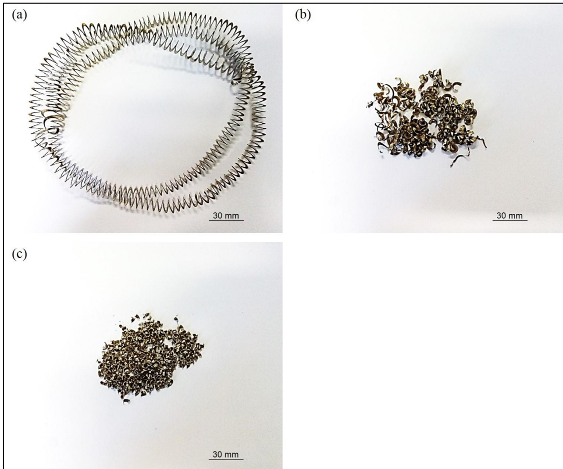
Figure 2. Chip forms. (a) Washer-type helical chip (reference tool); (b) Arc chip (chip-breaker model A); (c) Arc chip shorter than previously (chip-breaker model B)
