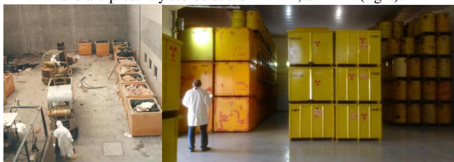
Figure 1: Waste collected in the state of São Paulo was conditioned in stainless steel boxes (left) and are presently stored at the RWMF, at IPEN (right).
