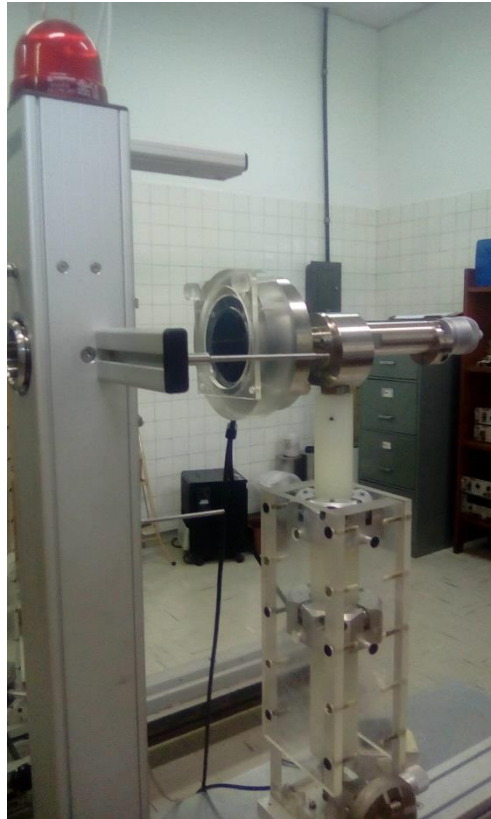
Figure 2. Extrapolation chamber entrance window covered by a Hostaphan absorber sheet.
