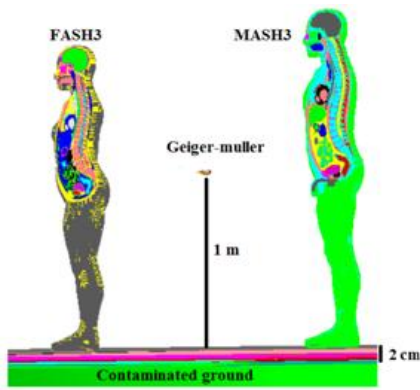
Figure 1. Exposition scenario with the FASH3 and MASH3 phantoms placed on contaminated soil.
