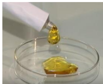
Fig. 1 - Hydrogel gel of PVP with silver nanoparticles for wound dressing.
