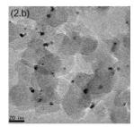
**Fig. 1.** Chronoamperometry comparing different samples. Fig. **2.** (a) TEM\_ Pt/CeO2 calcined at 400°C. (b) TEM\_ Pt/C.
