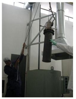
Figure 1. Charging of the reactor vessel inside the pit furnace
