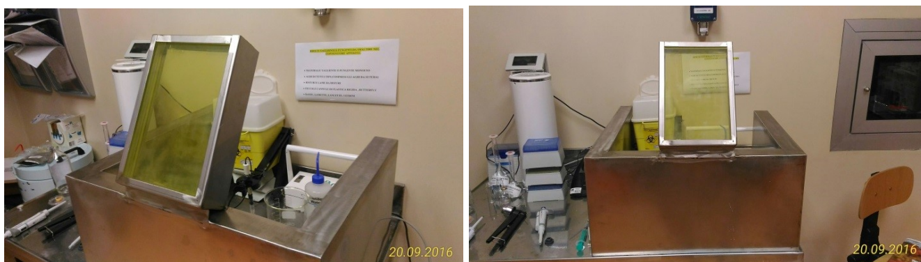
FIG. 5. Example of an inexpensive lead-shielded area for the manipulation of QC samples.
