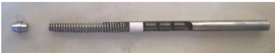
Fig. 1 – Typical actual fuel rod sectioned for visualization of the internal parts. At the left side one can see the end plug whose the lathe machining generates chips like the ones used in this paper.
