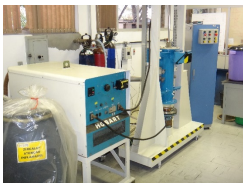
Fig. 5a – Actual image of the modified CCTM VAR Furnace.
